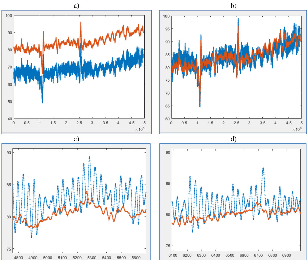
Figure 2.1 Comparison of BTTP heading (red) and compass heading (blue)
